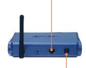
2. Connect the Power Adapter to the Access Point and then to a power outlet.
